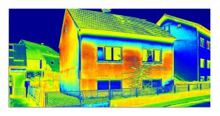
A thermal Infra red image of the outside of two houses. Blue is a cold outside wall; orange is a warm outside wall. The two houses adjacent to each other have notably different wall temperatures. The best insulated houses keep the warmth in and have cold outside walls. A thermal image shows where there are shortcomings in the insulation and which if addressed should reduce energy bills. The cost -effectiveness of improving insulation and how
